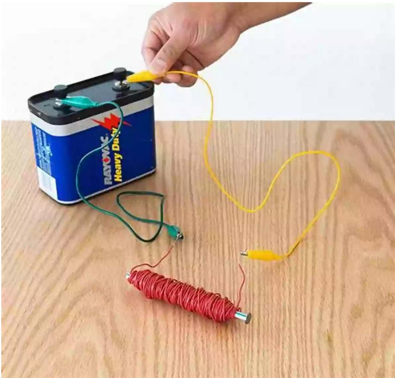
Explore the magnetic world by creating your own electromagnet using a battery, a nail, and insulated copper wire. Wrap the wire around the nail, leaving some wire ends exposed. Connect the ends to the battery and witness the nail becoming magnetized, attracting small metallic objects. This experiment introduces you to the principles of electromagnetism.
