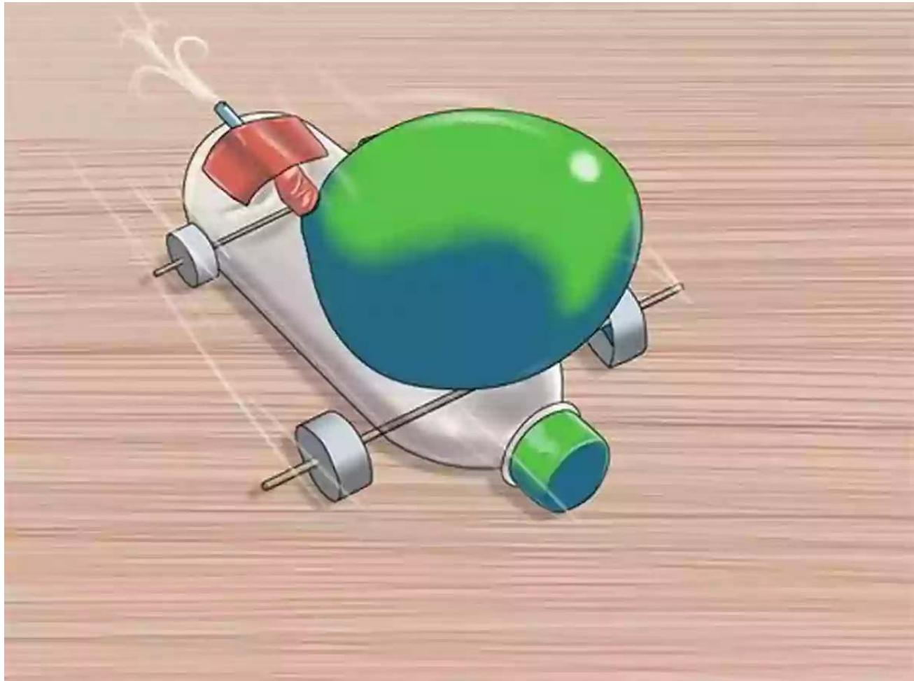
Construct a car that runs on the power of air by attaching a balloon to a small plastic bottle with wheels. Inflate the balloon and secure its opening, then release it to propel the car forward. This experiment allows you to explore Newton's Third Law of Motion while having a blast.
