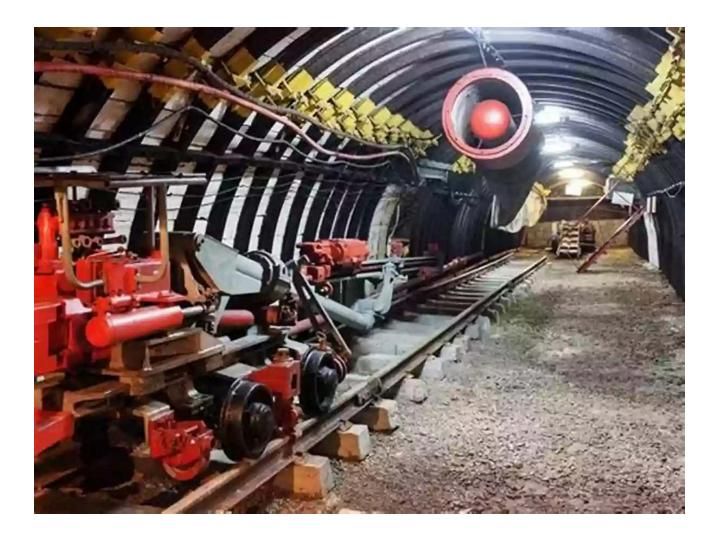
Mine ventilation is a vital aspect of the mining industry that ensures a safe and healthy working environment for miners. It involves the process of circulating fresh air throughout the mine, controlling airborne pollutants and preventing dangerous conditions such as gas build-up and excessive heat.
