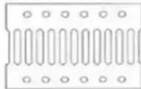
Figure 5. Slit steel damper at Art Hotel, Sapporo [9].
